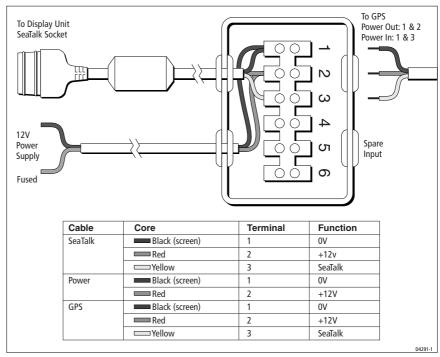
Figure 6-12: Using the Auxiliary Junction Box
